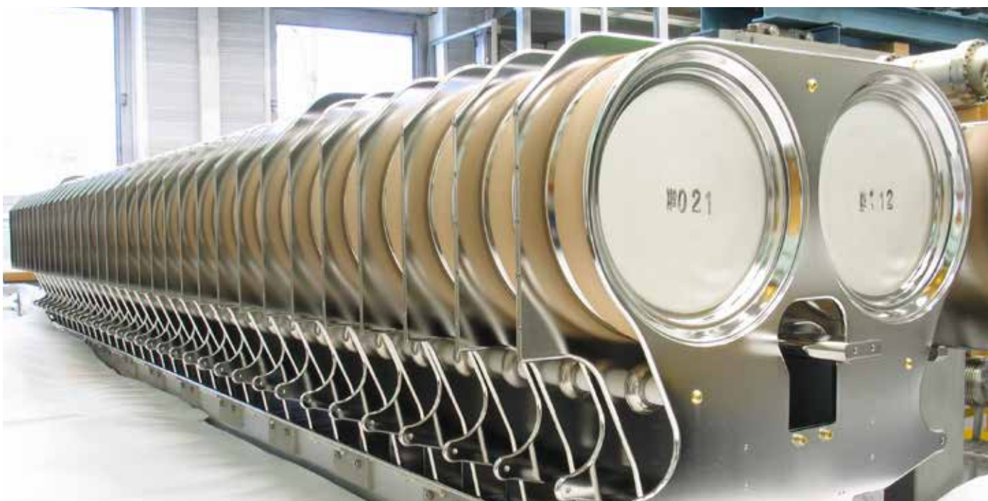
Assembly LHC Injection Kicker, CERN
