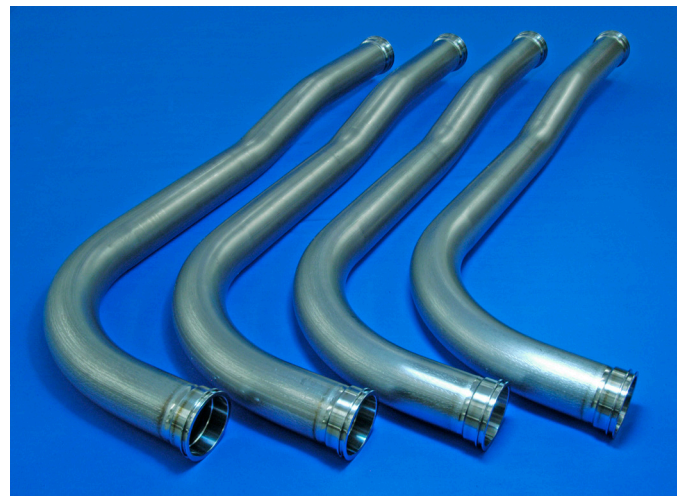
Titanium Tubes Wastewater system – AIRBUS
